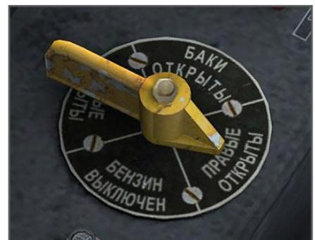
fuel system and allows no fuel to pass beyond the selector valve. The fuel selector is rotating clockwise with left click and anticlockwise with right click.
